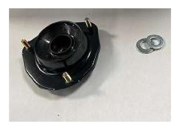
Take your factory upper mount and two 14mm washers and install them onto the strut as shown below.
