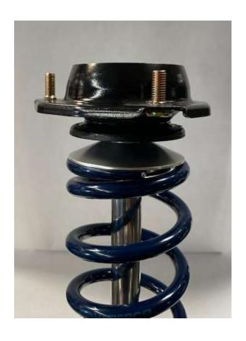
Once you are to this point, just spin the gold perch down and hold the shock shaft with a firm grip. Use an impact to tighten down the nylock till it is tight. Once that is done repeat the process on the other strut and install your coilovers.
