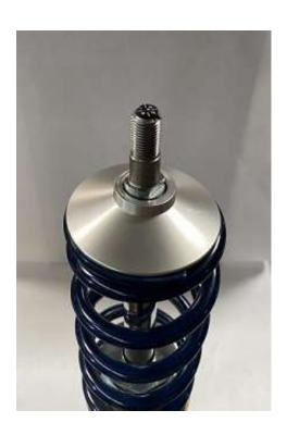
Start by removing the nut, washers, and spacers from the strut.
