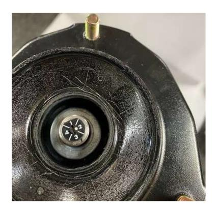
The top hat should just be resting on the conical hat with the two 14mm washers on the inside of the hat as shown.
