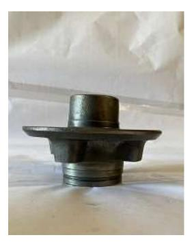
Once you've completely removed your factory brakes and have your bare hubs and spindle you will be ready to proceed.
