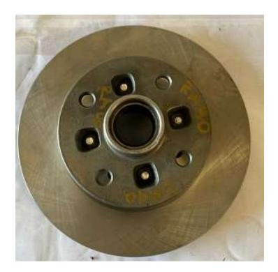
Bolt the rotor to the backside as shown above using the four 10x1.25x25mm bolts and lock washers.
