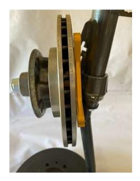
Install rotor and hub assembly onto the spindle, Install the greased outer bearing and torque according to manufacturer's specification or your preferred method, be sure to install a new cotter pin, and don't forget the dust cap.
