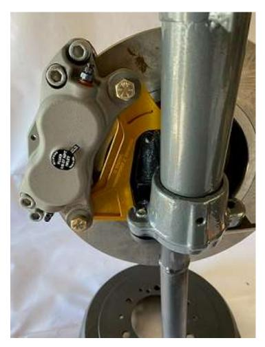
Slide the Caliper over the rotor and align the bolt holes on the bracket. Install the two  $3/8-24x1\frac{1}{4}$ " bolts and lock washers and torque to 30ft/lbs.
