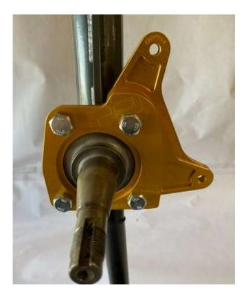
Start by bolting up the caliper bracket to the strut using the four 10x1.25x20mm bolts and lock washers as shown above.
