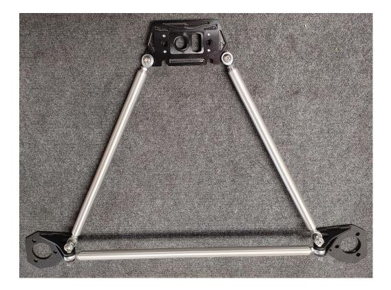
When you mount the two diagonal rods that go out to the strut towers, make sure that the rod ends on the bars sit below the clevis pin during the final assembly. Otherwise they can sit too tall and hit the hood. They should be configured as shown in the following pic.
