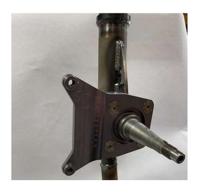
Install the bracket like shown using the four countersunk 10-1.25x20 bolts, torque to 35 ft/lbs.
