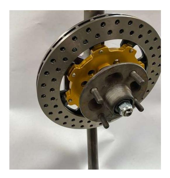
Install the hub with rotor and hat assembly onto the spindle, install the greased outer bearing and torque according to manufactures specification or your preferred method. Be sure to install a new cotter pin, and don't forget the dust cap.
