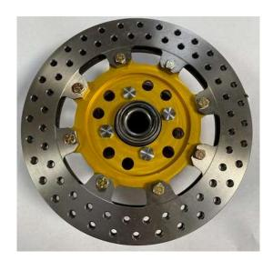
Place the rotor/hat assembly on the back side of your hub. Line up the bolt holes and install the four low profile 10-1.25x25 bolts by hand. Final torque to 35ft/lbs. If replacing/re-packing the wheels bearings, make sure to have the inner and outer races are installed, and the bearings packed with grease. Also be sure to have the inner bearing and seal installed.
