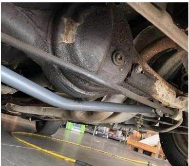
Once you have it all bolted up and looking correct it's time to eyeball the centering of the axle before taking it to get professionally aligned. Measure the wheel to the fender and
