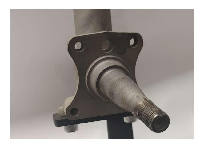
Remove factory brakes and backing plate until you have a bare spindle like shown above.
