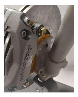
Slide the caliper over the rotor and bracket. Install two 3/8-24x1.25 hex head bolts with lock washers. Torque to 30 ft/lbs.
