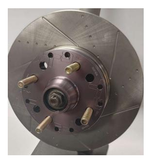
Slide the rotor onto the spindle, install the packed outer bearing, install keyed washer, spindle nut and related hardware. Follow manufacturer recommended procedure for torquing spindle nut.
