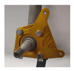
Install brackets onto strut casing using four M10-1.25x25 hex head bolts and lock washers noting correct right and left side placement. Brake caliper ears should face forward. Torque to 40 ft/lbs.
