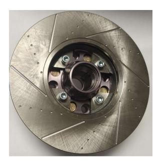
Slide the rotor over the back of the hub and install the four M10-1.25x35 Socket cap bolts with lock washers. Torque to 45 ft/lbs.
