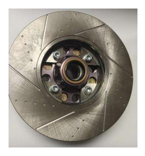
Your kit also includes new wheel bearings and hub seals. Pack the bearings and add grease to hub. Install packed inner wheel bearing and drive seal into place.
