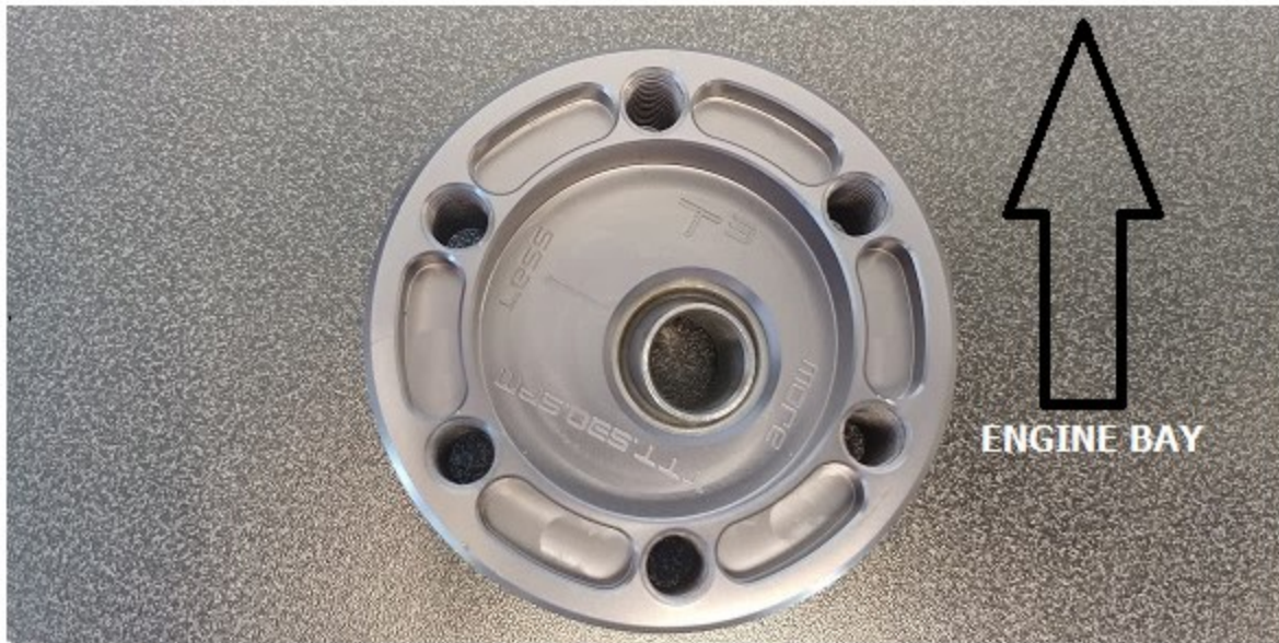
Position 3: Positive camber with positive caster
