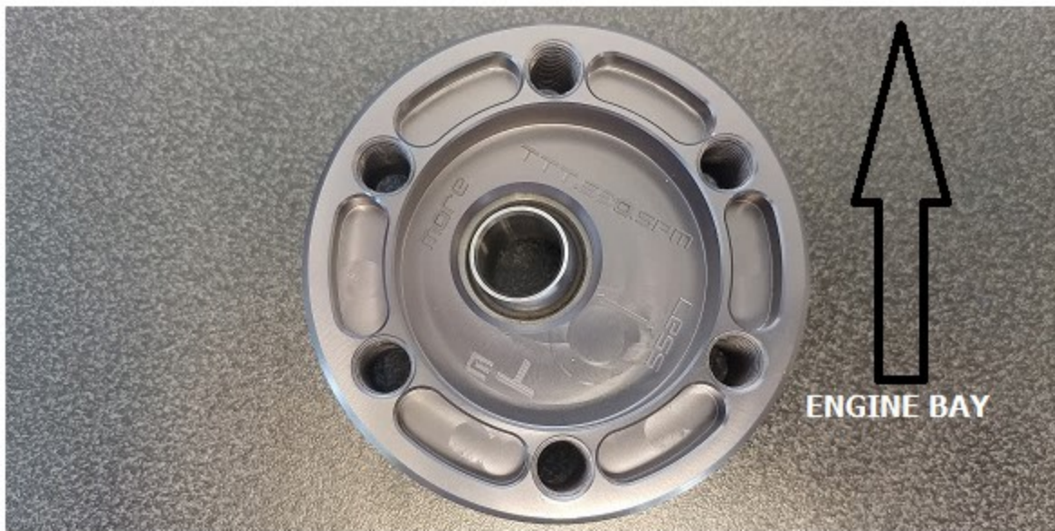
Position 6: Negative camber with negative caster
