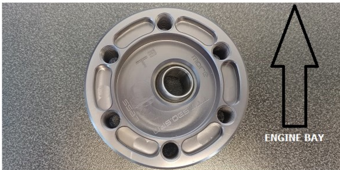
Position 2: Negative camber with positive caster
