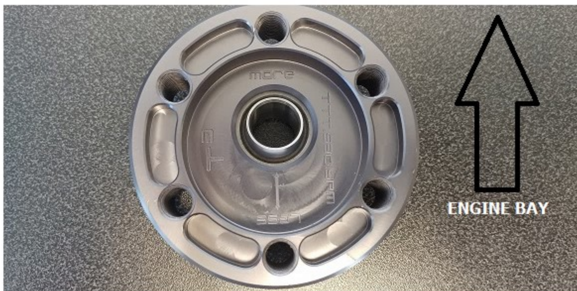
Position 1: Most negative camber position
