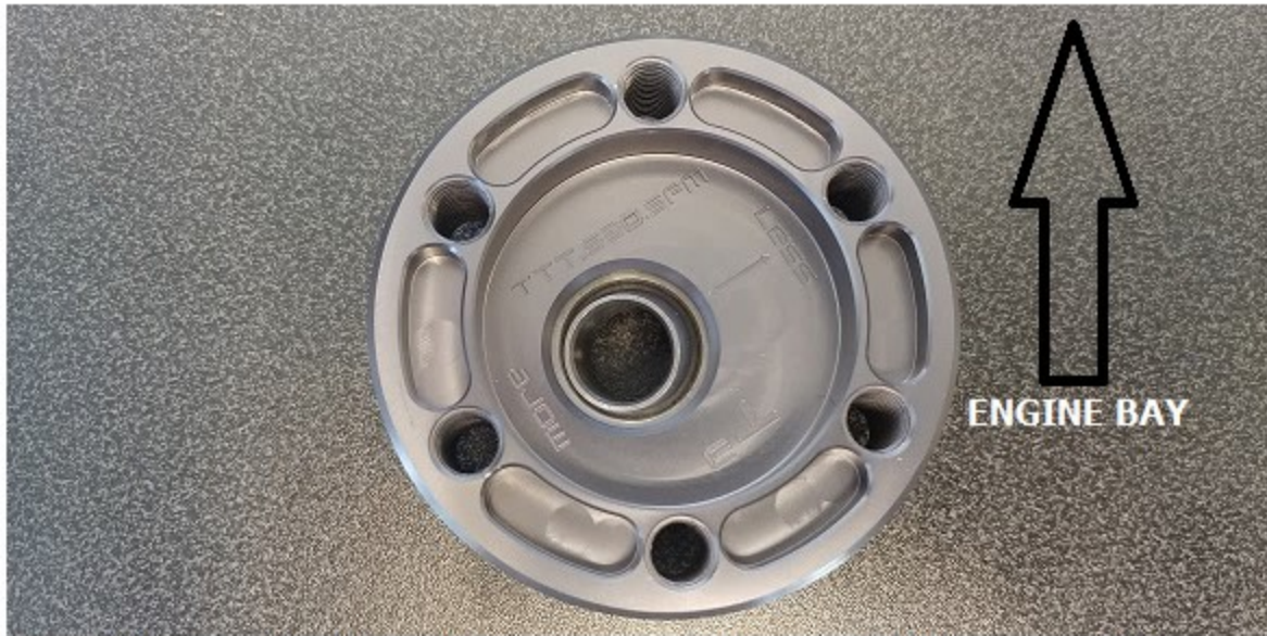
Position 5: Positive camber with negative caster
