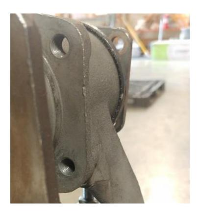
Remove factory drum brakes and all related parts until you have a bare mounting flange with 4 threaded holes. You can remove the stub axles and remove the backing plate (reference your repair manual for wheel bearing installation) or take the plate loose and cut them off with a cutoff wheel, plasma cutter, etc....
