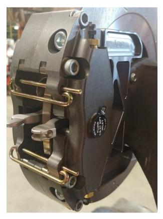
Slide the caliper over the rotor and install the two 3/8 shank bolts through the caliper and into the bracket and tighten to 35 ft/lbs.
