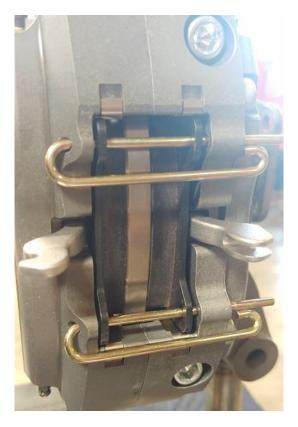
Slide out the retaining pins and install the pads than re-install the retaining pins like shown.
