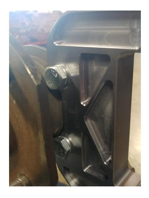
Install the bracket opposite of the strut tube onto the flange with the flatter side facing out, and the deeply recessed part facing the mounting flange. Torque the two 10mm shank bolts with lock washers to 45ft/lbs.
