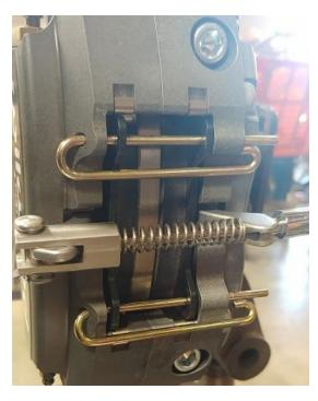
If you have the kit with parking brake function, install the cable as shown.
