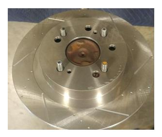
Slide the rotor over the wheel flange.
