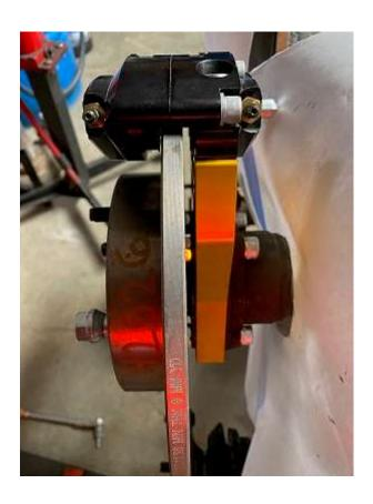
Place caliper onto bracket using the two 3/8-24x2 socket head bolts. Final torque 30ft/lbs.
