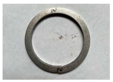
Halfmoon shims are placed Infront of bearing between caliper bracket and flange. Photo shown below. Shims are used to hold bearing tight in place once whole assembly is installed.
