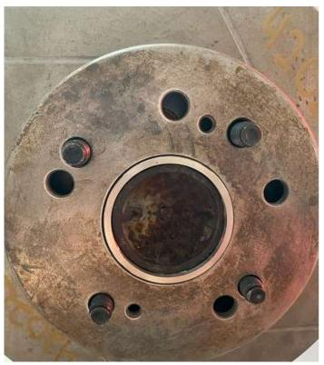
Add rotor alignment ring into rotor and slide over studs. Hand tighten a couple lug nuts on just to keep the rotor snug while finishing assembly.
