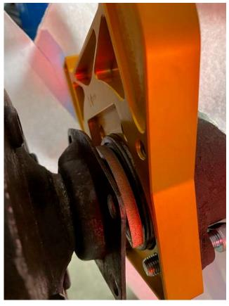
Once shims are connected all around, bolt flange and bracket together clamping whole assembly together. Final torque to 45ft/lbs
