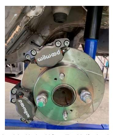
Once all completed the kit should fit up like this if using the wildwood set up.
