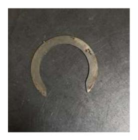
Halfmoon shims are placed in front of the bearing between caliper bracket and flange. Photo shown below. Shims are used to bearing tight in place once whole assembly is installed.
