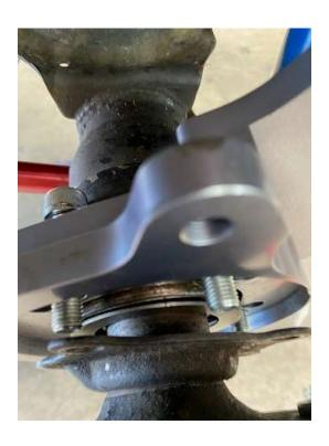
Once shims are put in place, Bolt flange and bracket together, clamping whole assembly together. Final torque to 45ft/lbs.
