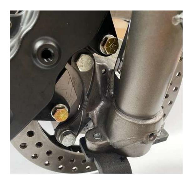
Slide the caliper and bracket over the rotor and align bolt holes on the bracket to the ones on the spindle. Torque down the two 12-1.25x25 bolts with lock washers to 60ft/lbs.
