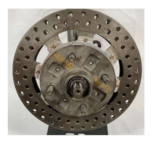
Install the hub with rotor and hat assembly onto the spindle, install the greased outer bearing and torque according to manufacturers specification or your preferred method. Be sure to install a new cotter pin, and don't forget the dust cap.
