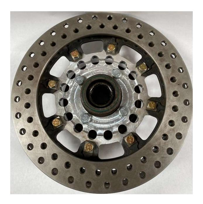
Place the rotor/hat assembly on the back side of your hub. Line up the bolt holes and install the four 10-1.25x25mm bolts by hand. Final torque to 35ft/lbs. If replacing/repacking the wheel bearing, make sure to have the inner and outer races installed, and the bearings packed with grease. Also be sure to have the inner bearing and seal installed.
