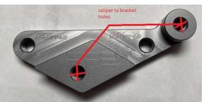
Once all bolted up in the correct orientation, torque down the 7/16-20x1.25 bolts to 40ft/lbs.
