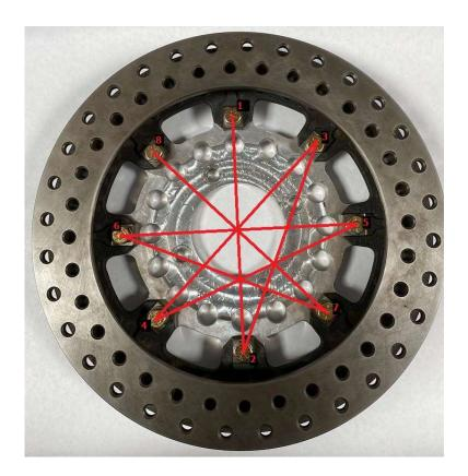
Place the rotor on top of the hat with the flat side facing down as pictured. Hand tighten the eight 5/16-18x1" bolts through the rotor and into the rotor hat in an alternating pattern as shown, and final torque to 24ft/lbs.
