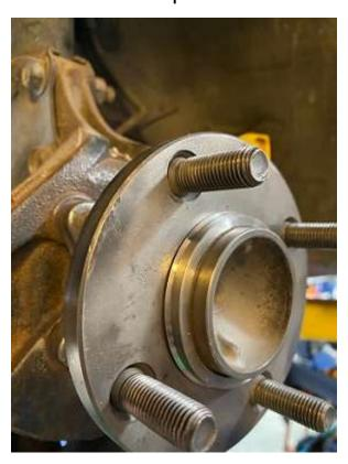
Install the rotor alignment ring as shown.
