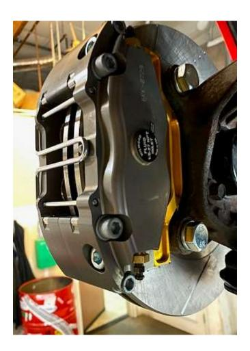
Slide the caliper over the rotor and align bolt holes on the bracket. Install the two 3/8-24x1¾ allen head bolts and milspec washers.
