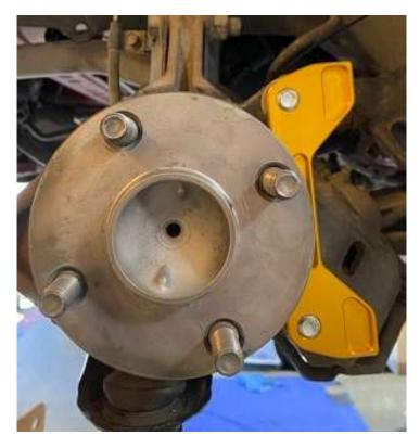
Install the as shown using the two 12-1.25x30mm bolts and lock washers. Torque to 60ft/lbs.
