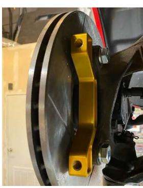
Install the rotor onto the hub assembly. Snug the lugs up by hand to hold the rotor in place.
