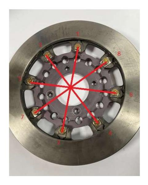
Place the rotor on top of the hat with the flat side facing down as pictured. Hand tighten the eight 5/16-18x1" bolts through the rotor and into the rotor hat in an alternating pattern as shown, and final torque to 24 ft/lbs.
