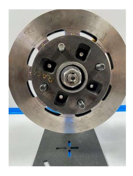
Install the hub with rotor and hat assembly onto the spindle, install the greased outer bearing and torque according to manufacturers specification or your preferred method. Be sure to install a new cotter pin, and don't forget the dust cap.
