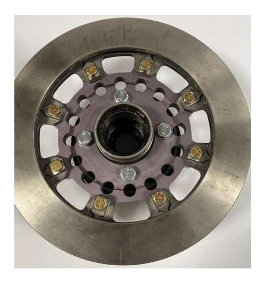
Place the rotor/hat assembly on the back side of your hub. Line up the bolt holes and install the four 10-1.25x30mm bolts by hand. Final torque to 35 ft/lbs. If replacing/re-packing the wheel bearings, make sure to have the inner and outer raced installed, and the bearings packed with grease. Also be sure to have the inner bearing and seal installed.
