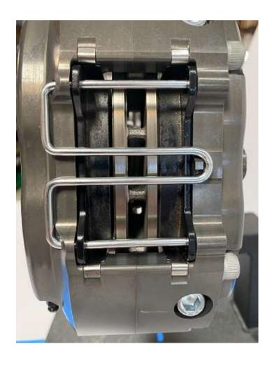
Slide the caliper over the rotor and align bolt holes of bracket. Install the two 3/8-24x2" bolts and torque to 30 ft/lbs.
