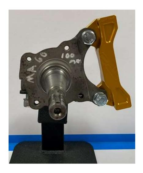
Install the bracket like shown using two 12-1.25x25 bolts and lock washers. Torque to 60ft/lbs.
