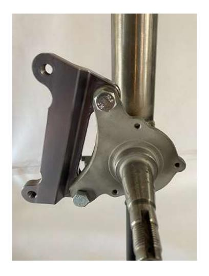
Start by installing the Caliper bracket to the spindle with the two 10x1.25x30mm bolts and lock washers as shown above.
