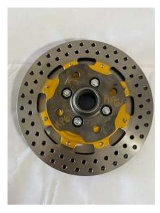
Place the rotor/hat assembly on the back side of your hub. Line up the bolt holes and slip the four 10x1.25x30 bolts though the hat and up and hand tighten the 10mm flange nuts to the bolts on the back side of the hub.
