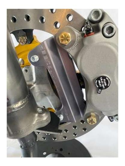
Slide the Caliper over the rotor and align the bolt holes on the bracket. Install the two 3/8-24x1.25" bolts and lock washers and torque to 35ft/lbs.
