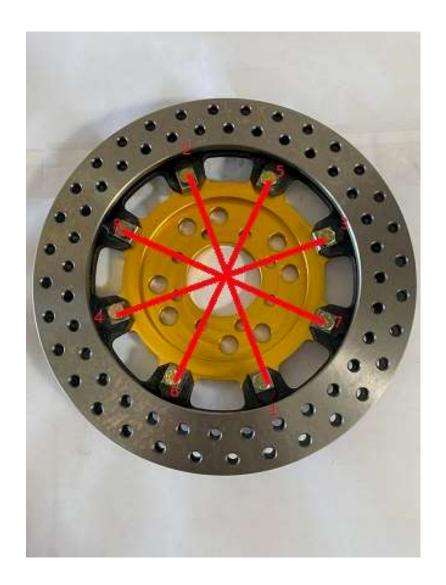
Place the rotor on top of the hat with the flat side facing down as pictured. Hand tighten the eight 5/16-18x1" bolts through the rotor and into the rotor hat in an alternating pattern as shown, torque to 24ft/lbs.
