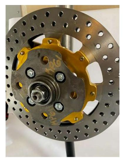
Install the hub with the rotor and hat assembly onto the spindle, install the greased outer bearing and torque according to manufacturers specification or your preferred method. Be sure to install a new cotter pin, and don't forget the dust cap.
