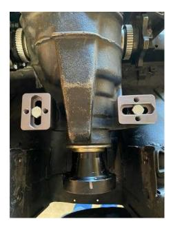
Orient the blocks as shown and bot them to the differential using the two 12x1.75x100mm bolt and flange nut. Torque to 50ft/lbs.
