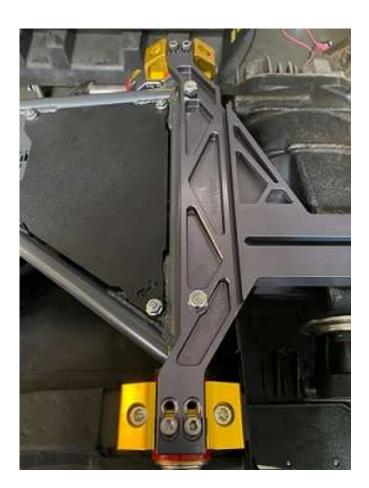
Align the eight 8x1.25x20mm allen head bolts up with the wholes of the fancy caps and bolt the power brace to the fancy cap. Torque to 30ft/lbs.
