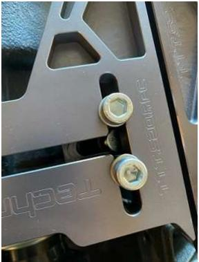
Bolt the power cradle to the to the blocks using the four 10x1.25x40mm Allen head bolts and Milspec washers. Torque the bolts to 30ft/lbs.
