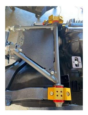
To being installing the power cradle, install the fancy caps first using the eight 10x1.25x35mm Allen Head bolts in place of the old factory control arm caps.
