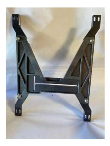
Bolt the power brace to the cradle using the four 10x1.5x40mm Button heads and nylocks.
