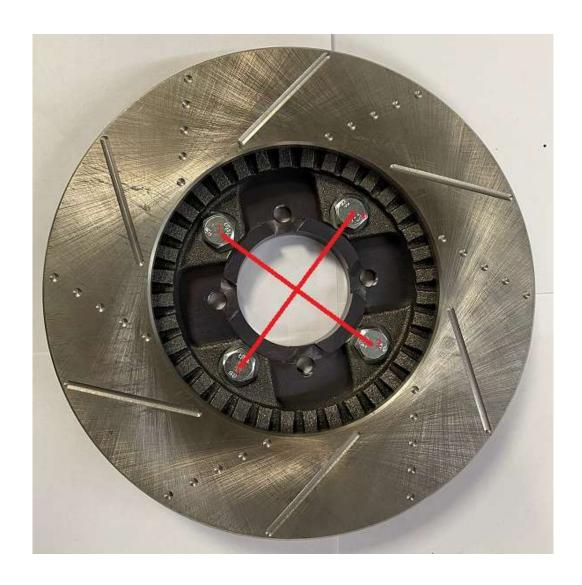
Place the rotor on top of the hat with the flat side facing down as pictured. Hand tighten the four 10-1.25x20 bolts through the rotor hat in and alternating pattern as shown, and final torque to 45ft/lbs.
