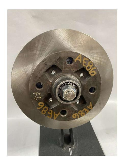
Install the hub with rotor and hat assembly onto the spindle, install the greased outer bearing and torque according to manufactures specification or your preferred method. Be sure to install a new cotter pin, and don't forget the dust cap.
