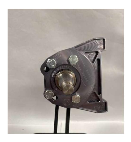
Install the bracket as shown using the four 10-1.25x25 bolts and lock washers. Torque to 45ft/lbs.
