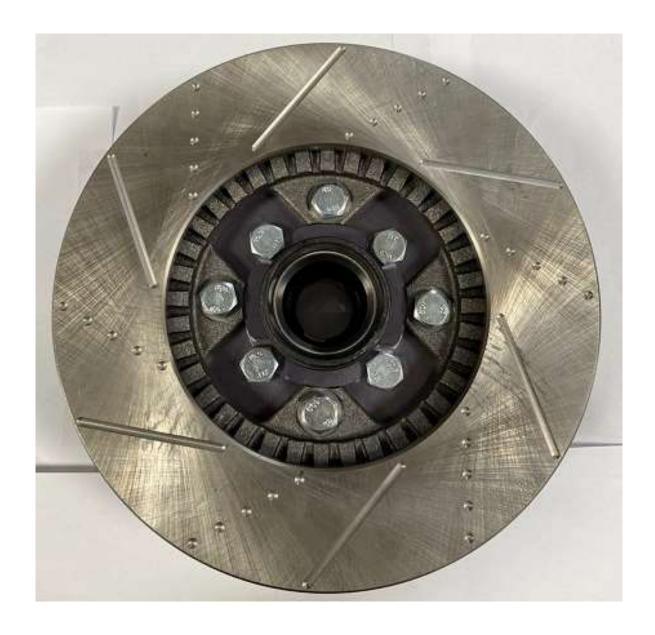
Place the rotor/hat assembly on the back side of your hub. Line up the bolt holes and install the four 10-1.25x25mm bolts by hand. Final torque to 45ft/lbs. If replacing/re-packing the wheel bearings, make sure to have the inner and outer race installed, and the bearing packed with grease. Also be sure to have the inner bearing and seal installed.
