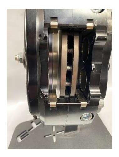
Slide the caliper over the rotor and align the bolt holes of the bracket. Install the two 10-1.25x45 socket head bolts and torque to 30ft/lbs.
