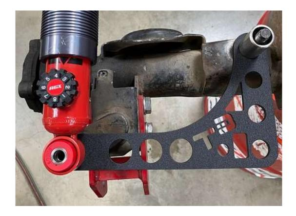
Install shock on the shock tab and install 10mm spacer into shock bushing and install 20mm spacer onto lateral rod pin as shown above.
