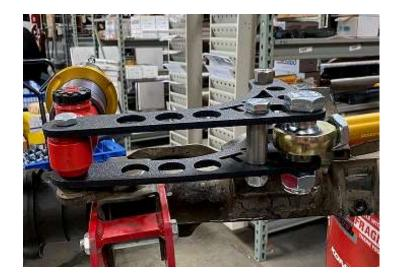
Select one of the three holes that puts lateral rod closest to factory angle.
