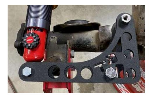
Install second half of drop mount with the 10mm bolt hole on the shock side. Install 10-1.25x25 bolt, Datsun and 12-1.25x70 bolt as shown above.
