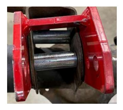
Install the 12-1.25x90 bolts through the 12mm spacers and bolt them down. Final torque to 65ft/lbs.
