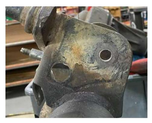
Slide the traction bracket over bare bracket with the hump on the same side as the shock tab.
