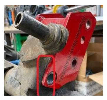
Once the traction bracket is slid into place install the large and small tubes through the flange and traction bracket.
