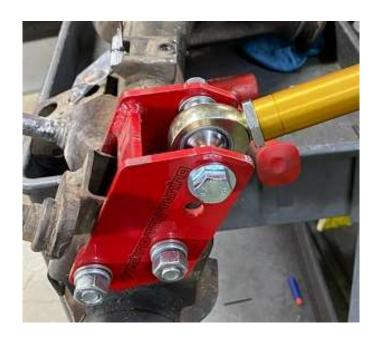
Once you have one side completed move to the next side and repeat the process. (Once all bolted up make sure pinion angle is as close to factory as possible)
