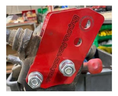
Once you have the traction bracket torqued into place all that is left if putting the links back onto either one of the two holes on the end of the traction bracket.
