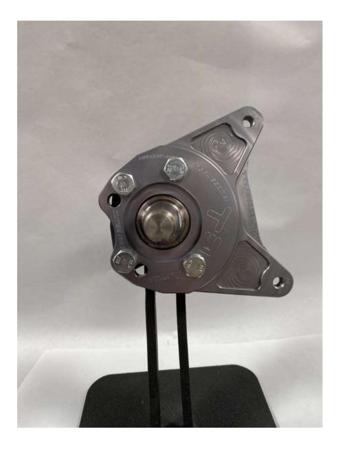
Install the bracket like shown using four 10-1.25x25 bolts and lock washers. Torque to 45ft/lbs.
