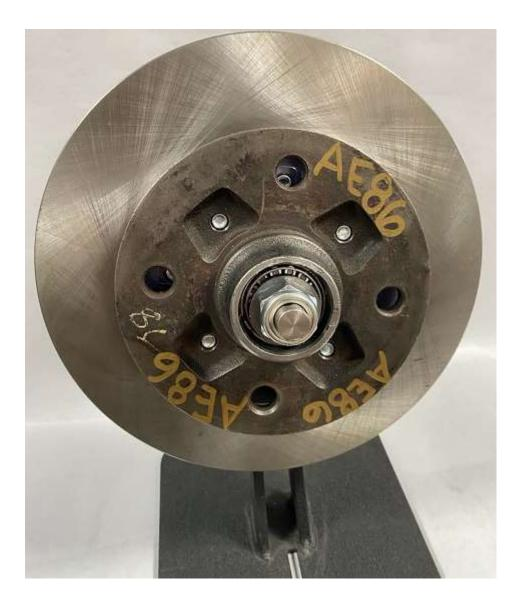
Install the hub with rotor and hat assembly onto the spindle, install the greased outer bearing and torque according to manufactures specification or your preferred method. Be sure to install new cotter pin, and don't forget the dust cap.
