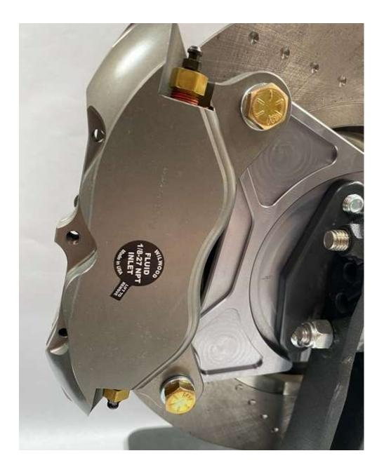
Slide the caliper over the rotor and align bolt holes of bracket. Install the two 3/8-24x1.25" bolts with lock washers and torque to 30ft/lbs.
