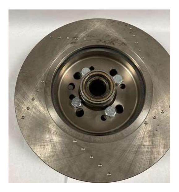
Place the rotor on the backside of your hub. Line up the bolt holes and install the four 10-1.25x25mm bolt by hand. Final torque to 45ft/lbs. If replacing re-packing the wheel bearing, make sure to have the inner and outer race installed, and the bearing packed with grease. Also be sure to have the inner bearing and seal installed.
