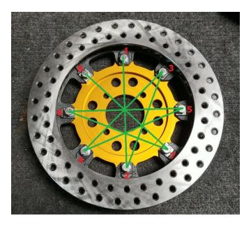
Place the rotor hat with the plain side facing up as pictured and the flat side of the rotor facing down as pictured. Hand tighten all bolts with lock washers through the rotor and into the hat in an alternating pattern as shown. Final torque to 24 ft/lbs.
