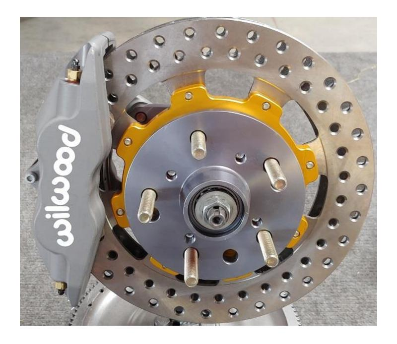
Repeat this process for the other side, thread the 90-degree elbows into the calipers until snug and facing the appropriate direction to allow brake hoses to clear, thread the brake hose onto both ends and snug down. Bleed the brakes as outlined in your repair manual, double check for any leaks, and your all set!
