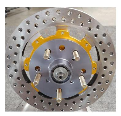
Install the hub with rotor assembly onto the spindle, push the outer bearing into place, install the plate washer and hand thread the spindle nut on. Torque nut according to the specification outlined in your repair manual, and be sure to use a new cotter pin.
