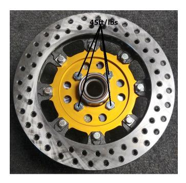
Place the rotor with hat assembly onto the hub, align holes and Install the four 10mm bolts with lock washers through the hat and into the hub, hand tighten in an alternating pattern and torque to 45 ft/lbs. If replacing/re-packing wheel bearings, make sure inner and outer races are installed, and bearings are packed with grease. Also please be sure to have inner bearing in place as well as the seal installed and lightly grease lip of seal.
