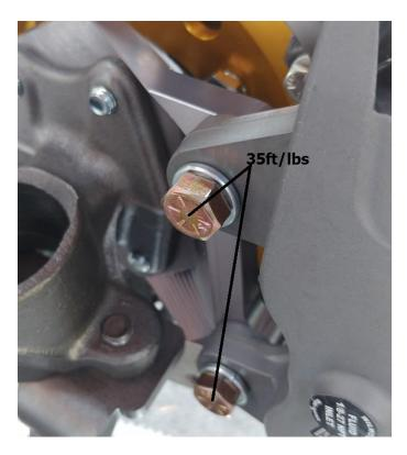
Slide the caliper over the rotor and align the holes with the bracket, thread the two bolts with lock washers through the caliper and into the bracket and torque to 35 ft/lbs.
