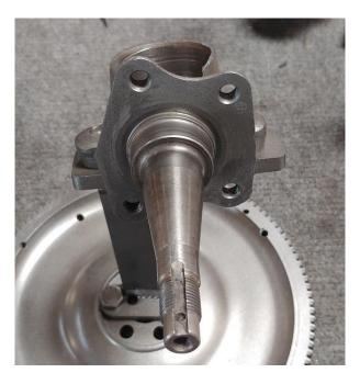
Remove factory brakes until you have a bare spindle like shown above.
