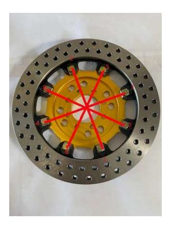
Place the rotor on the top of the hat with the flat side facing down as shown. Hand tighten the eight 5/16-18x1" bolts through the rotor and into the rotor hat in an alternating pattern as shown.
