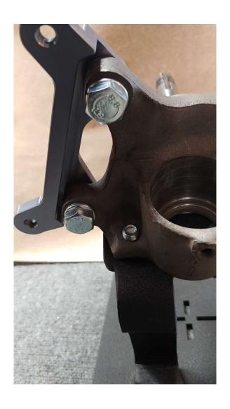
Start by installing the Caliper Bracket to the spindle with the two 12x1.25x35mm bolts and lock washers as shown above Torque bolts to 45ft/lbs.
