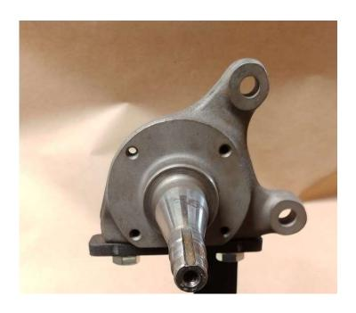
Once you have completely removed your factory brakes and have your bare hubs and spindles you will be ready to proceed.
