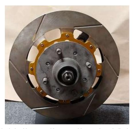
Install the hub with rotor and hat assembly onto the spindle, Install the greased outer bearing and torque according to manufacturers specification or your preferred method. Be sure to install a new cotter pin, don't forget the dust cap.
