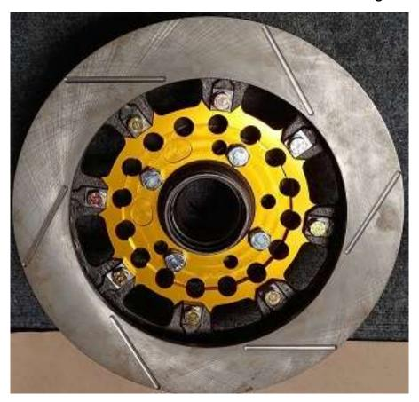
Place the rotor/hat assembly on the back side of your hub. Line up the bolt holes and install the four 10-1.25x25mm bolts and lock washers by hand. Final torque to 35ft/lbs. If replacing/re-packing the wheel bearing, make sure to have the inner and outer races installed, and the bearings packed with grease. Also be sure to have the inner bearing and seal installed.
