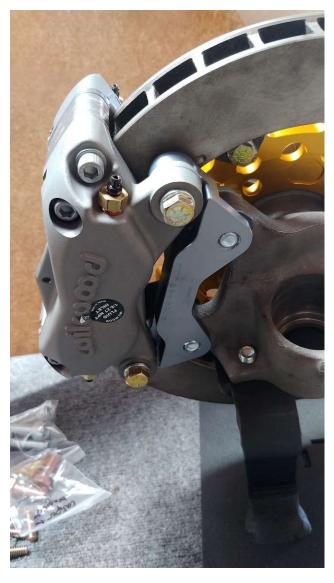
Slide the caliper of the rotor and align the bolt holes on the bracket. Install the two 3/8-24x1.25" bolts with lock washers and torque to 30 ft/lbs.
