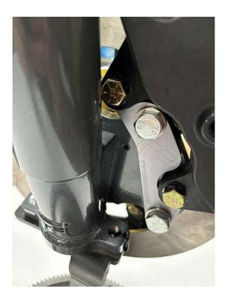
Slide the caliper and caliper bracket over the rotor and align the bolt holes to the ears on the spindle. Install the two 12x1.25x40 AH bolts with lock washers and torque to 65ft/lbs.
