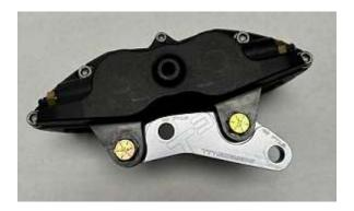
Start by installing the caliper bracket to the caliper using the two 7/16x20x1.25" bolts and lock washers and torque to 40ft/lbs.
