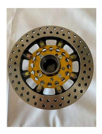
Place the rotor/hat assembly onto the backside of the hub. Line up the bolt holes and install the four 10x1.25x30 bolts into the hub. Final torque to 35ft/lbs. for 10mm bolts. (Five 12x1.25x30 if using our five lug billet hubs), Final torque to 42 ft/lbs. If replacing/repacking the wheel bearings, make sure to have the inner and outer races installed, and the bearings packed with grease. Also be sure to have the inner bearing and seal installed.
