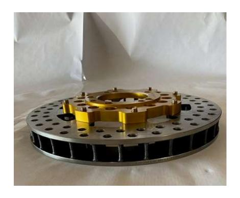
Rotor and Rotor Hat should look as shown when completed.
