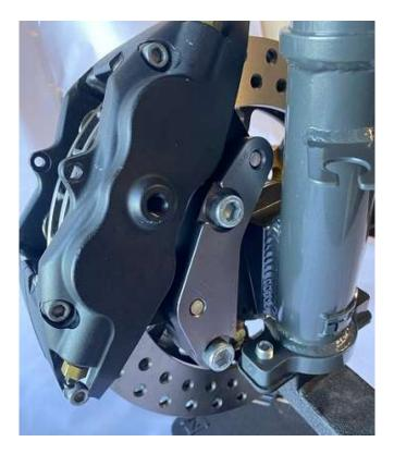
Slide the caliper and caliper bracket over the rotor and align the bolt holes to the ears on the spindle. Install the two 12x1.25x40 AH bolts with lock washers and torque to 65ft/lbs.
