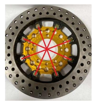
Next Install the rotor hat to the rotor.
