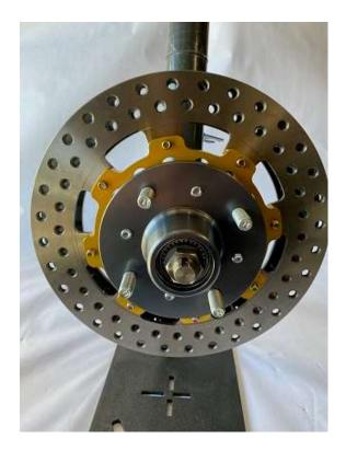
Install the hub with rotor and hat assembly onto the spindle, install the greased outer bearing and torque to manufactures specifications or preferred method. Be sure to install new cotter pin, and don't forget the dust cap.
