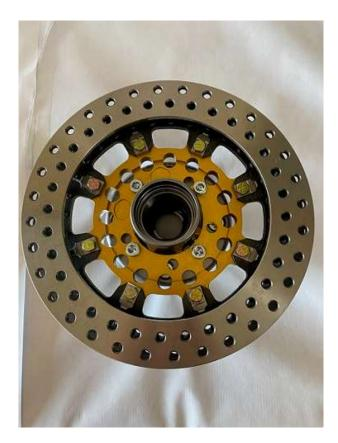
Place the rotor/hat assembly onto the backside of the hub. Line up the bolt holes and install the four 10x1.25x30 bolts into the hub. Final torque to 35ft/lbs. for 10mm bolts. (Five 12x1.25x30 if using our five lug billet hubs), Final torque to 42 ft/lbs. If replacing/repacking the wheel bearings, make sure to have the inner and outer races installed, and the bearings packed with grease. Also be sure to have the inner bearing and seal installed.
