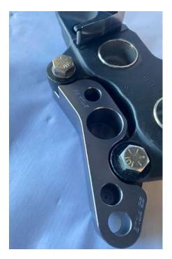
Start by installing the caliper bracket to the caliper using the two 7/16x20x1.25" bolts and lock washers and torque to 40ft/lbs.
